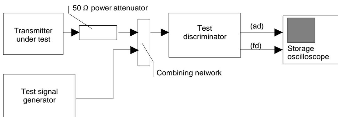
**Figure 3: Measurement arrangement**
